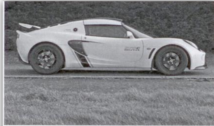
Figure 11.2 Lotus Exige 270E tri-fuel – able to run on any mixture
